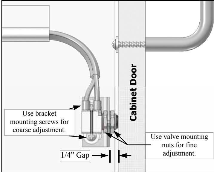
First determine a height location where the pilot/actuator valve is to be mounted on the inside of the cabinet opposite the door hinge, preferably about knee height or higher. The objective is to mount the pilot/actuator valve so that the inside face of the cabinet rests against the button of the pilot/actuator valve. This will set the door ajar very slightly, about 1/32".
