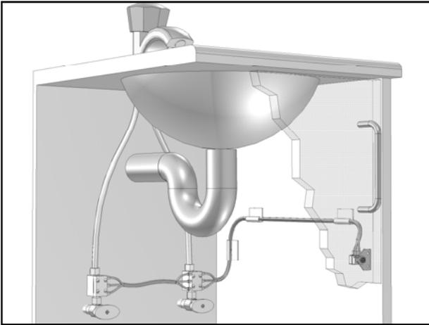
This illustration shows a typical installation for the Model 1720 Tapmaster. The valve blocks are connected in-line on the hot and cold water supplies with 3/8" O.D. compression fittings. The pilot/actuator valve is mounted about knee height on the inside wall of the cabinet opposite the door hinge. The control tubing is routed in between the valves. Water flow to the faucet is activated by pressing with the knee or leg against the cabinet door.
