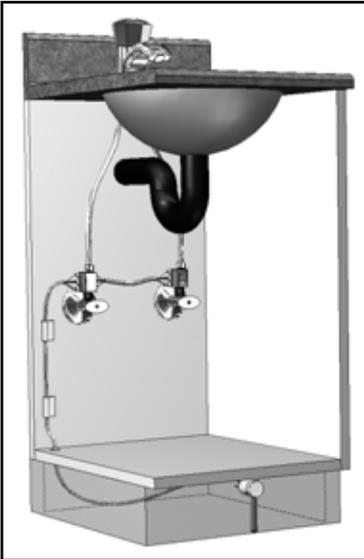
This illustration shows a typical installation for the Euro Model 1770 series Tapmaster. The valve blocks are connected in-line on the hot and cold water supplies with 3/8" compression fittings. The Euro foot activator is mounted on the cabinet toe kick with the control tubing routed from the foot activator through the cabinet base to the hot and cold water supplies to make the connections to the valve blocks.
