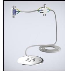
This illustration shows a typical Model 1780 Tapmaster. The valve blocks connect in-line on the hot and cold water supplies with 3/8" O. D. compression fittings. The pilot/actuator valve is mounted to the underside of the activator disk which is mounted to the floor with the three #8 countersunk screws provided.
