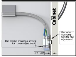
First determine a height location where the pilot/actuator valve is to be mounted on the inside of the cabinet opposite the door hinge, preferably about knee height or higher. The objective is to mount the pilot/ actuator valve so that the inside face of the cabinet rests against the button of the pilot/ actuator valve. This will set the door ajar very slightly, about 1/32".
