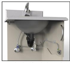
connected in-line on the hot and cold water supplies with 3/8" O.D. compression fittings. The pilot/actuator valve is mounted about knee height on the inside wall of the cabinet opposite the door hinge. The control tubing is routed in between the valves. Water flow to the faucet is activated by pressing with the knee or leg against the cabinet door.
