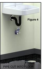
simpler to drill or core one hole at the activator disk location and another to permit access into the wall behind you and the sink. A "U" shaped piece of conduit or plastic pipe (depending on local codes) could be installed to allow the control tube bundle to be fished through underneath the sink. This example is only one of many possible solutions to route the control tube bundle.
