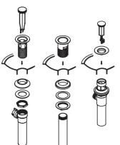
**6.** Place a ring of plumbers putty on the bottom of the flange and apply Teflon tape on the threaded tailpiece. Thread tailpiece to the drain body. Insert flange through drain hole and attach drain body to the flange from under the sink.
