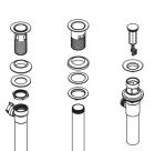
**5.** Remove flange from drain body.
